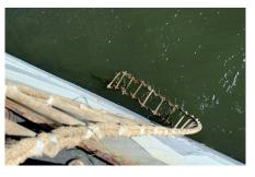
barges, various supply boats, etc.) while alongside the main vessel. Jacob's ladders are preferred as they are lighter and easy to carry (average weight of a pilot ladder is approx. 88 kg whilst jabob's ladder is around 17 kg.) than the pilot ladders, although latter is much more safer.
